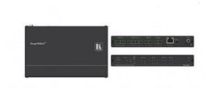
The FC-28 is a PoE-powered control gateway, capable of plug and play deployment over customer Ethernet LAN for remote control of customer controlled devices via bidirectional RS-232, IR, GPI/O and relay control connections. Multiple control clients can be IP-connected to the FC-28 control gateway for concurrent control of two RS-232, four IR controllable devices, such as AV scalers, video displays, audio amplifiers, DVD players, sensors, screens, shades, door locks, and lighting
